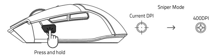
Customize the Sniper Mode's DPI or remap the Multi-Function Trigger for other tasks using Razer Synapse.
